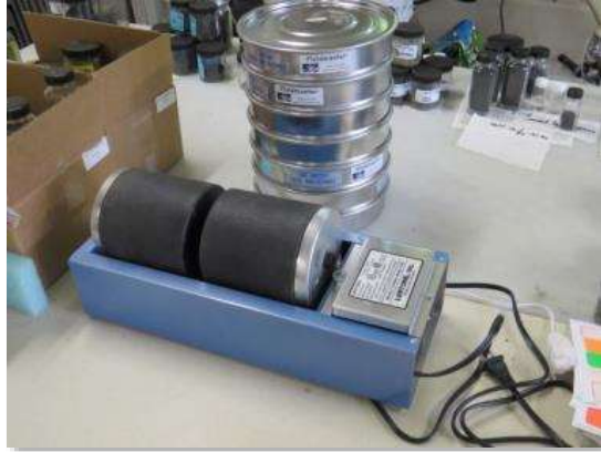
Figure 552 – Mixing and reducing the sediment
