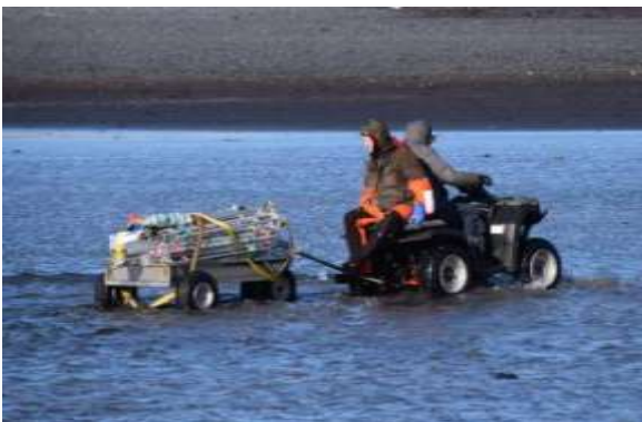
Figure 80 – The ATV was able to operate on flooded terrain.
