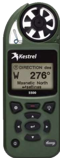
Figure 105 – The Kestrel weather station
